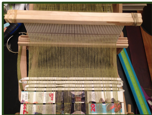
Above: Position for warping a Schacht 10" rigid heddle loom (that lacks support for a second heddle) Below: Schacht Cricket set up for fine tabby at 24 ends per inch. Both heddles are tied together at the top and move as one unit.
