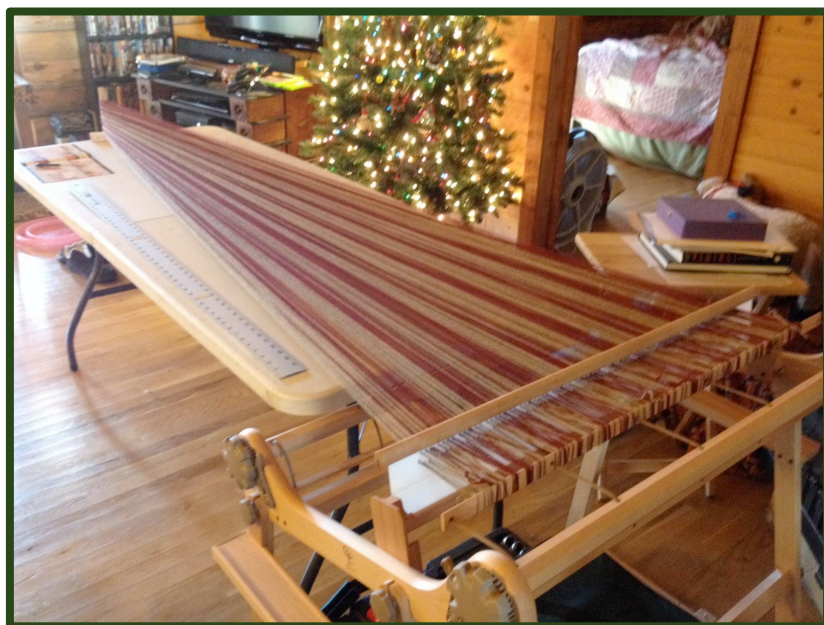
Above: A rigid heddle loom set up to warp directly onto the beam using a peg system.
