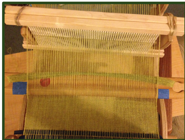
Above: Blue painters tape on the shuttle allow me to regularly check, and adjust, the width of the textile as needed.
