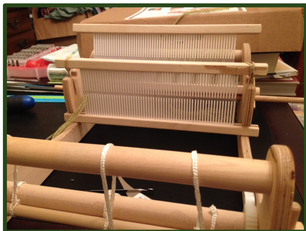
Above: Position for warping a Schacht 10" rigid heddle loom (that lacks support for a second heddle) Below: Schacht Cricket set up for fine tabby at 24 ends per inch. Both heddles are tied together at the top and move as one unit.
